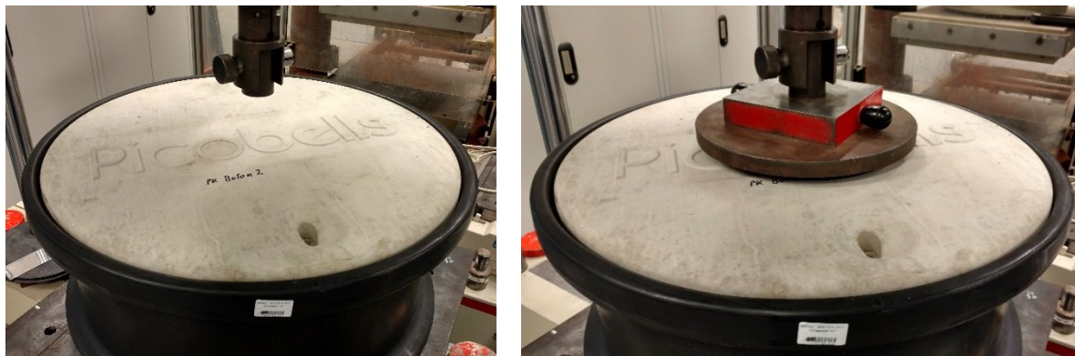
Fig. 1: Concrete cover „Picobells 200 kg“ Fig. 2 Test stamp d = 250 mm, rubber interlayer
